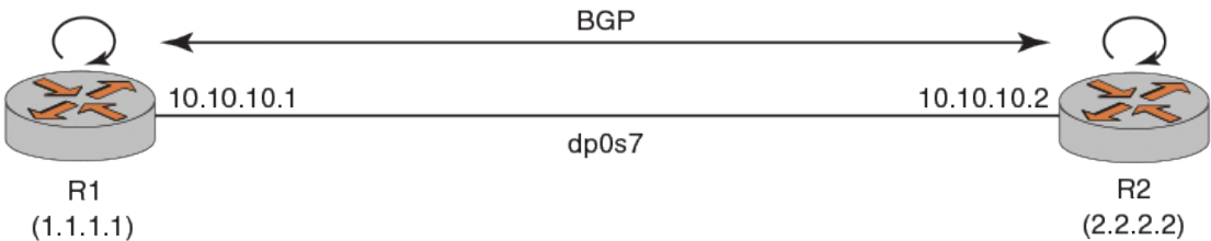
FIGURE 4 Configuring BFD for BGP single hop by using IPv4 addressing
